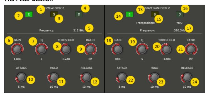
The Filter Section has the EQ and Dynamics control for each Octave band and each Resonant Filter band. Each band has an EQ with a gain control and a bandwidth control. Each band also has a dynamics processor with the standard threshold, ratio (from and expander at a 0.5 to 1 ratio up to a hard limiter at infinity to 1), attack and release controls as well as a hold control.
