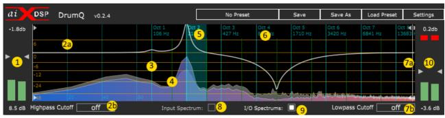
The *Spectrum Display* shows frequency vs level as well as the current state of all the Filter Bands. Here you can also work with general functions, like input and output levels.
